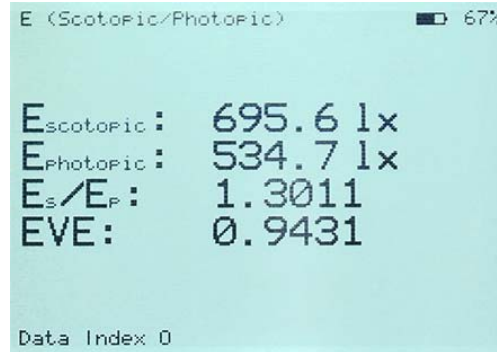
Relationship between the scotopic and photopic illuminance and the EVE factor as per IES TM-24-13
