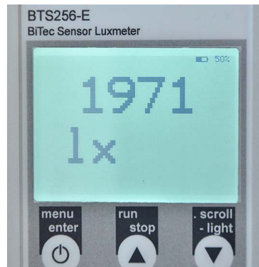
BTS256-E for illuminance measurement
